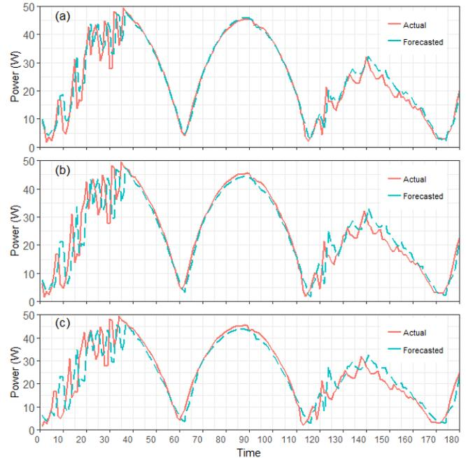
Fig. 4. Observed against forecasted AC power for: (a) 10 minutes, (b) 30 minutes and (c) 60 minutes forecasts. The night hours are filtered out.
