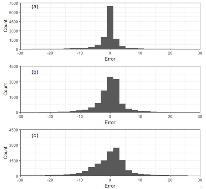
Fig. 3. Error histogram of: (a) 10 minutes, (b) 30 minutes and (c) 60 minutes forecasts. The histogram demonstrated a scattered variation moving from 10 to 60 minute forecasting.
